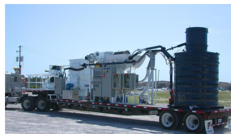
Trailer-mounted furnace for Transportable Waste-to-Energy System
